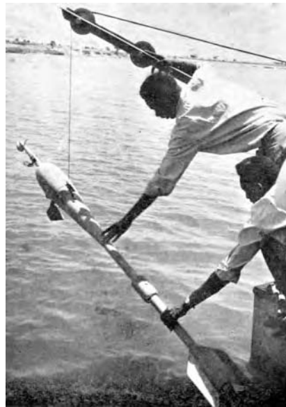
Fig. 4.10 Propeller-type Current Meter — Neyrtec Type with Sounding Weight
