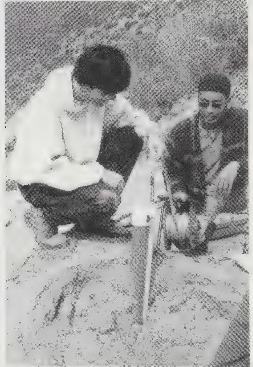
Figure 3.22 Using an electronic probe to measure the water level inside an observation well. When the electrodes on the bottom of the tape touch the water, an electrical circuit is closed and a buzzer sounds inside the reel. Also see Figure 7.7.
