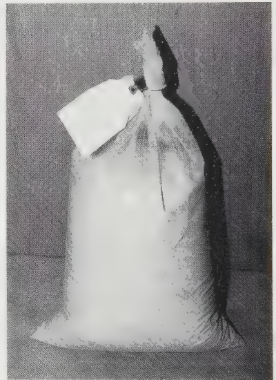
Figure 3.17 A typical disturbed sample stored in a plastic bag. The label attached to the bag identifies the sample.
