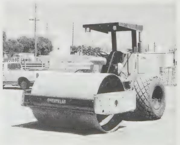
Figure 6.22 Self-propelled vibratory roller.
