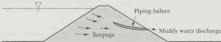
Figure 15.6 Piping failure in an earth dam.
