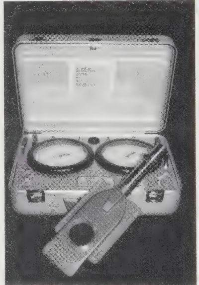
Figure 3.34 The Marchetti dilatometer with its control unit and nitrogen gas bottle. (Courtesy GPE, Inc., Gainesville, FL).
