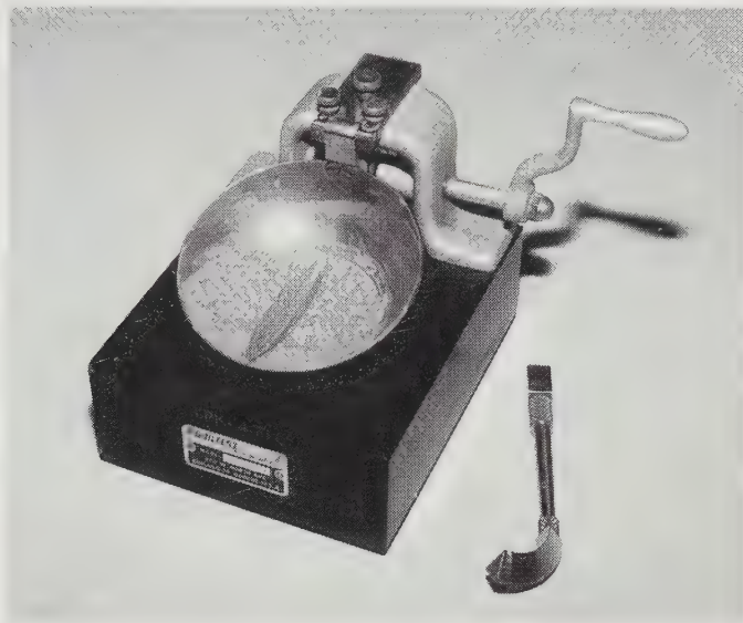
Figure 4.18 This device is used to perform the liquid limit test. The soil pat is in place and has been grooved with the grooving tool shown on the right. The next step is to begin turning the crank, which will repeatedly drop the cup.
