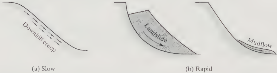
Figure 2.27 Colluvial soils: a) Slowly formed by creep; b) Rapidly formed by landslides or mudflows.
