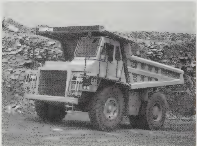
Figure 6.15 A large dump truck. This one is too large to travel on highways, and is used only when all of its movement can occur off road. Smaller dump trucks also are available, and they can travel on highways. (Caterpillar Inc.)
