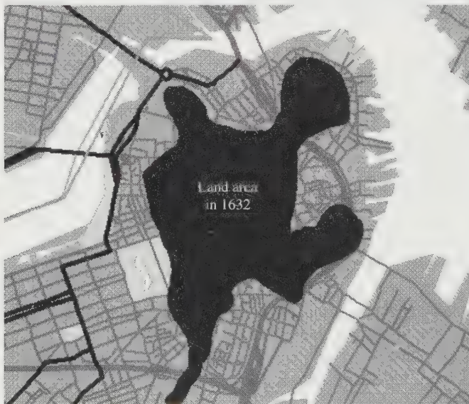
Figure 2.23 When the Puritans first settled in Boston, Massachusetts, the land area was as shown by the black zone in this map. It was connected to the mainland via a narrow isthmus. Since then, the city has been extended by placing fill in the adjacent water, thus forming the shoreline as it now exists.
