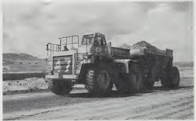
Figure 6.16 A very large off-road wagon. Upon reaching its destination, this wagon will unload the soil through doors on the bottom. Smaller versions of this design can be towed by semi tractors over the highway.
