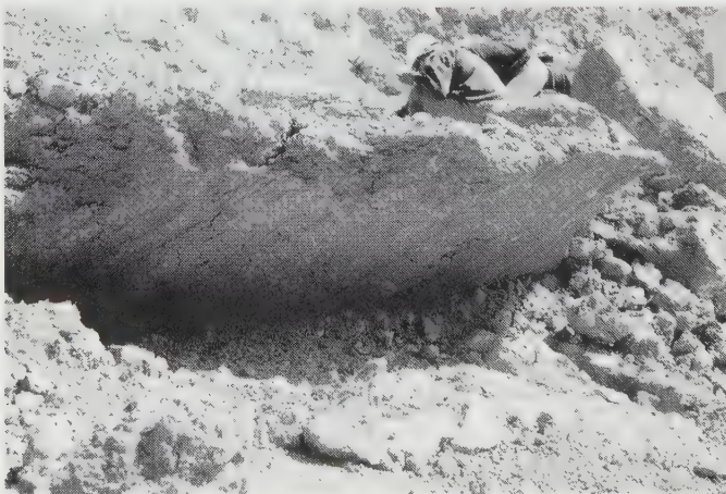
Figure 13.22 This slickenside was formed by a landslide in a clay. The shear strength along this surface has been reduced to the residual value.
