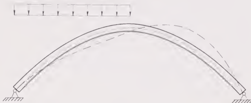
(b) Arch of same shape as (a) but subjected to different loading, which causes arch axis to bend into shape something like exaggeration shown by dashed line
