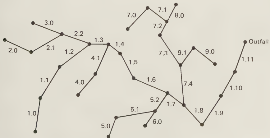
Fig. 2.2 Example key plan of a piped drainage system in an urban area
