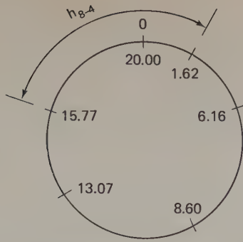
Figure 15.2. Definition of time gap between first and last vehicle in counting interval.
