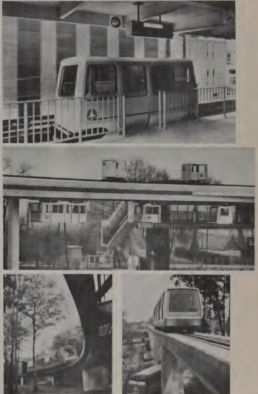
Figure 22.21. Types of AGT vehicles. SOURCES: U.S. DEPARTMENT OF TRANSPORTATION, Urban Mass Transportation Administration, Automated Guideway Transit Technology Overview , Washington, D.C., August, 1978. Advanced Transit Association International Conference, Advanced Transit and Urban Revitalization—An International Dialogue: Proceedings , Volume I, Indianapolis, Ind., 1978.
