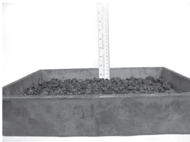
FIGURE 4.6 Mixture conditioning for volumetric mix design
