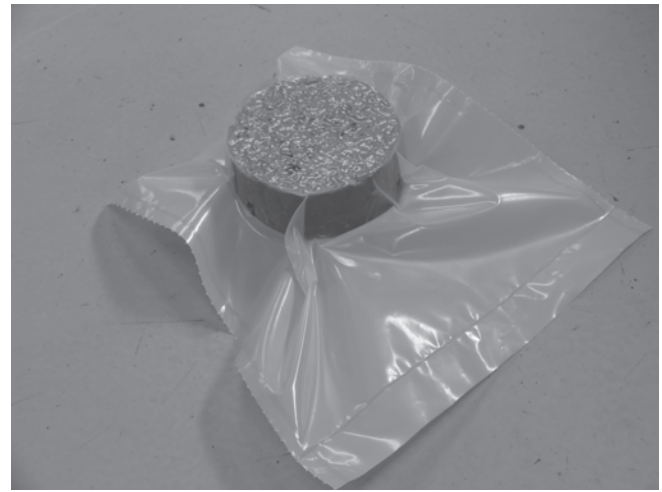
Figure 4.10 Asphalt Mix Sample in Sealed Bag
