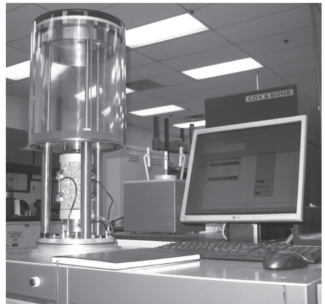
FIGURE 10.6 AMPT (Environmental Chamber Raised, Instrumented Specimen Loaded)
