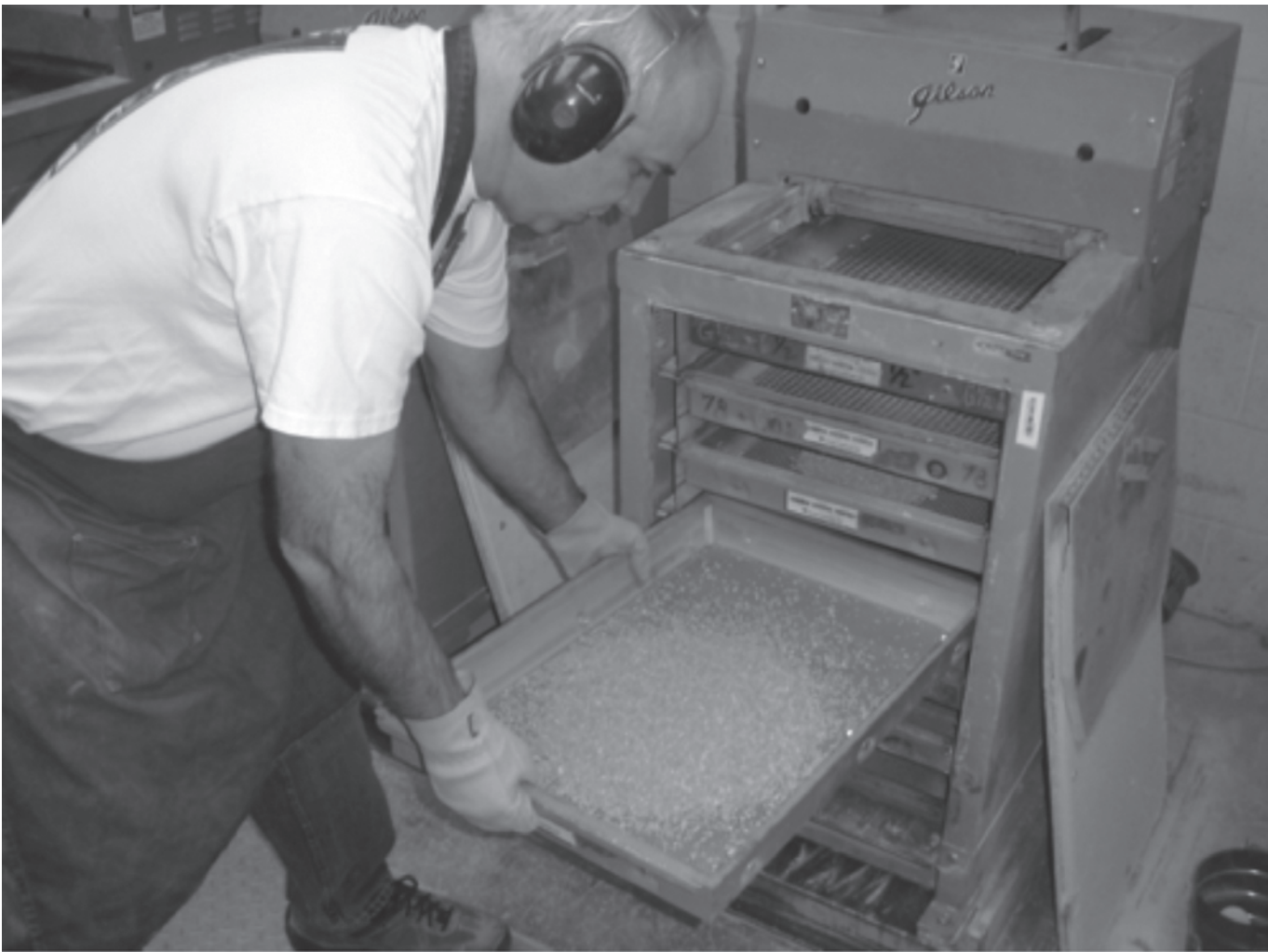
FIGURE 3.9 Fractionating aggregate on a large tray-type shaker
