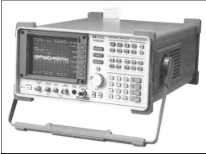
Figure 16.42 A typical spectrum analyzer. (Courtesy of Hewlett-Packard.)
