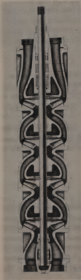
Figure 17.4 Deep-well multistage mixed-flow turbine pump. (Courtesy of Byron Jackson Company.)
