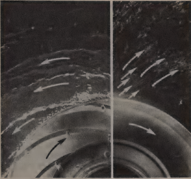
Figure 6.12 Radial-flow-pump impeller rotating at 200 rpm. (a) Instantaneous photo showing relative flow. (b) Time exposure showing absolute flow. (Photographs from Hydrodynamics Laboratory, California Institute of Technology.)
